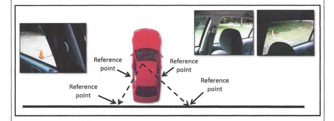
To determine when the rear of the vehicle is three feet away from a line when backing and turning, drivers can develop reference points. When a driver turns his/her head and looks over the right shoulder, he/she will see the line disappear in the rear window corner post. This is the point where drivers should begin turning the steering wheel when backing around a corner.
