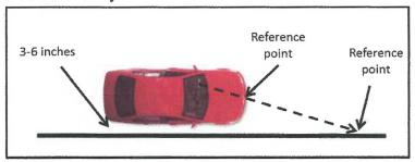
To determine when the right side of the vehicle is three feet from the curb or line, the line of sight reference is to align the right 1/4 section of the hood to the curb or the edge line of the roadway.
