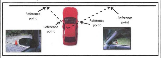
Drivers can develop reference points to determine when the front end of your vehicle is a few feet beyond the curb line and where you should begin to turn the steering wheel at intersections. The curb or line should appear to run under the driver side view mirror, and the driver can see where to go without the driver's vision cutting across the curb line. This is the point at which the driver should begin to turn the steering wheel to make the left turn.
